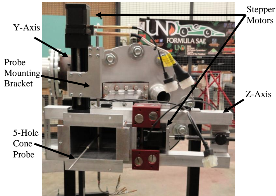
Figure 15. The five-hole cone probe traversing system used for exit velocity surveys during aerodynamic secondary loss testing.
