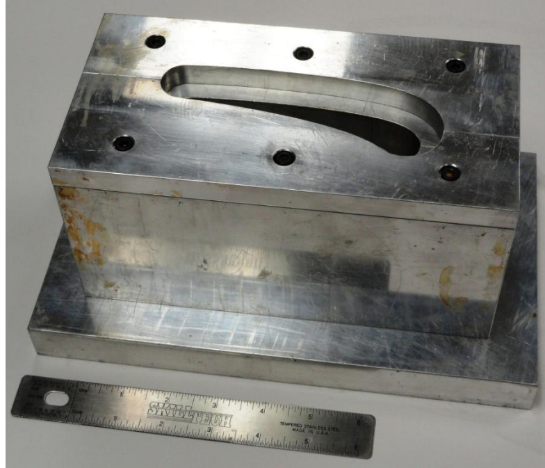
Figure 19. Aluminum mold used to cast the vane geometry from high temperature epoxy.
