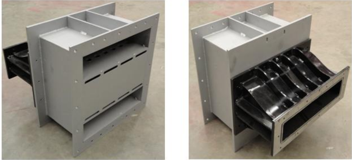
Figure 17. Images of the mock aero-derivative combustor turbulence generator.
